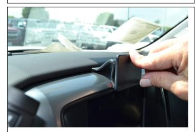
3. Press firmly forward on the ProClip so it flexes forward and the angled edge hooks around the panel frame edge under the padded part of the dashboard.
