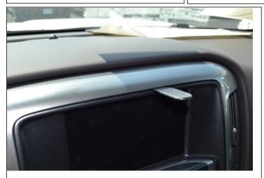
1. Press the thin end of the enclosed gap opener into the gap between the center console information screen panel and panel frame surrounding it, to widen the gap.
