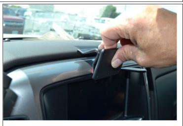
2. Place the ProClip in your hand so the ProClip label (sticker) is in an upright position, or if vertically positioned; the P in ProClip is at the top.
